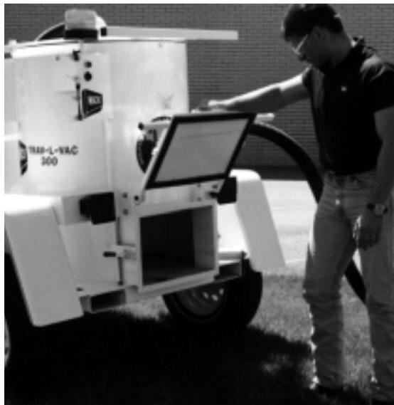
Figure 3-7. Open the dump gate to remove solid debris from the tank.
