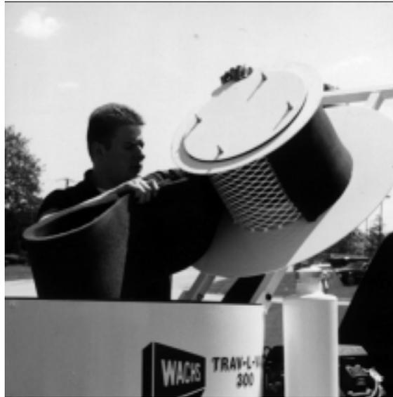
*Figure 3-8. Open the tank lid and clean the filter after each use.*
