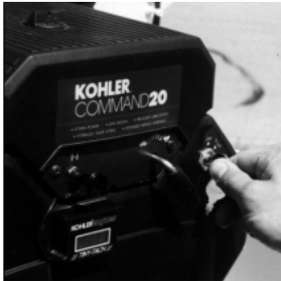
Figure 3-5. Use the key starter to start the engine.
